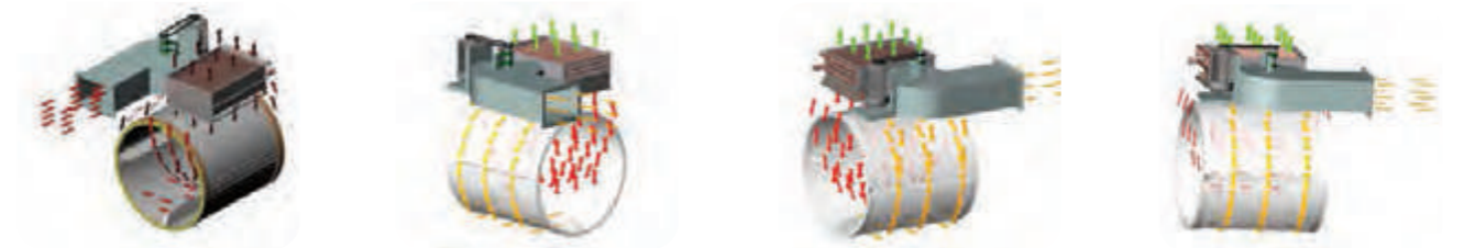
Heated Air Flow Circulation Diagram through the Steam Coil, Rotating Basket and extracted out by the suction Blows to the exhaust duct.
