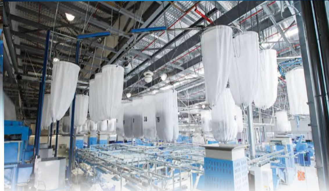
Bag storage and Loading system
