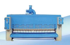
Using high-speed Image washer-extractors in combination with Image ironers improves the productivity and increases the quality. The most efficient way of removing moisture from linen is by high extraction and ironing. Our ironers are built to handle the linen direct from our washers.
