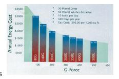
can even be taken straight from the washer-extractor to an ironer or finisher without slowing down the productivity. The high speed, or G-force, is the driving factor. By utilizing the inverter technology it has been possible to achieve this high-speed extraction in freestanding machines. The inverter automatically measures the out-of-balance electronically and decides if the machine can proceed to high speed, generating a high G-force.
