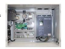
components such as contactors and relays. It provides a powerful yet simple drive alternative that is more economical than multi-motor drives. The inverter makes it possible to achieve high extract speeds and significantly save energy and time in the drying process. A multi-motor drive is optional.
