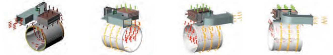
Heated Air Flow Circulation Diagram through the Steam Coil, Rotating Basket and extracted out by the suction Blows to the exhaust duct.
